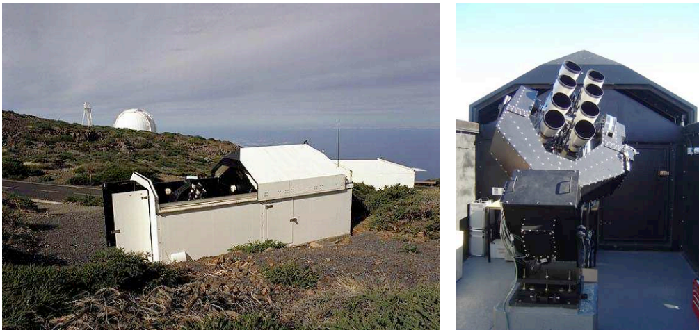
Figure 1.6: The SuperWASP observatories. Left: The enclosure of SuperWASP-N on La Palma. Right: The eight cameras of WASP-South in South Africa. Photographs taken from the SuperWASP website – http://www.superwasp.org
